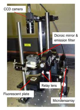
Fig.8 Fluorescence detection optical system
