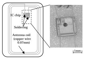
Fig.10 Laser soldering of antenna wire of IC card
