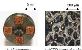
(a) Appearance (b) CCD image of surface Fig.6 cBN (325/400) grinding wheel with copper binder
