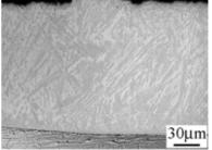
Fig.12 Microstructure of laser-alloyed intermetallic compound
