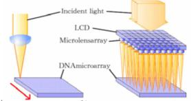
(a) Confocal laser scanning (b) LCD multi-spot fluorescent detection
