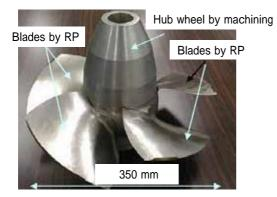
Fig.5 Stainless-steel bladed wheel built by SLS process (Courtesy Hitachi Corporation)
