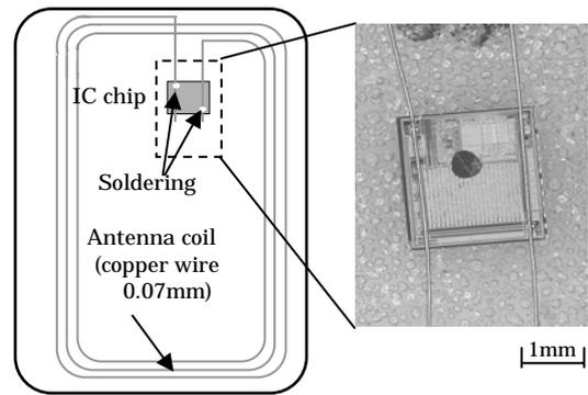
Fig.10 Laser soldering of antenna wire of IC card
