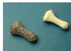
Fig.2 Fabricated bone and its base model
