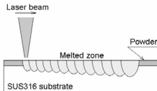
Fig.11 Schematic of laser surface alloying using powder
