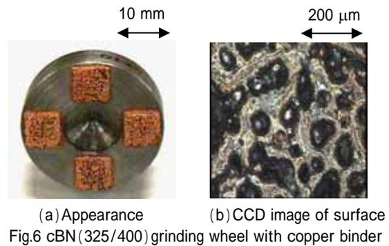
Fig.6 cBN(325/400) grinding wheel with copper binder
