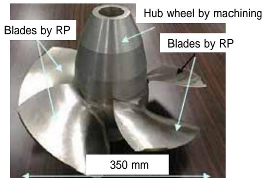
Fig.5 Stainless-steel bladed wheel built by SLS process (Courtesy Hitachi Corporation)
