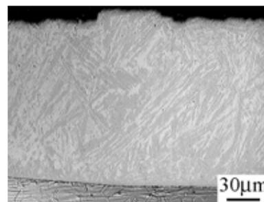
Fig.12 Microstructure of laser-alloyed intermetallic compound
