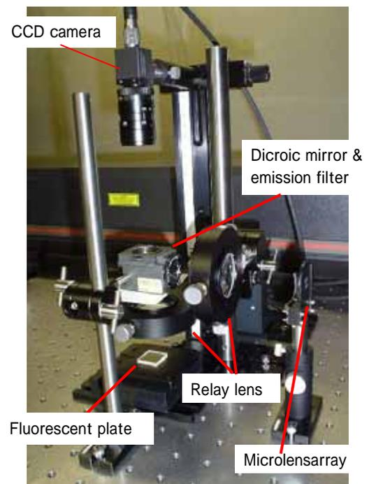
Fig.8 Fluorescence detection optical system
