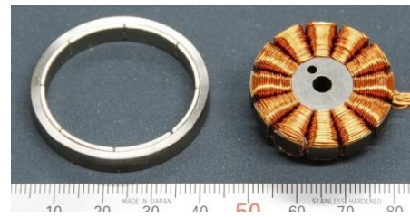
Fig. 2 Radial type self-bearing motor
