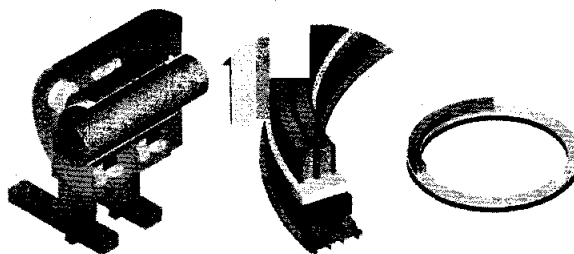
FIGURE 1: Topologies of the investigated SMB's: Radial bearing (left) and planar bearing (right)
